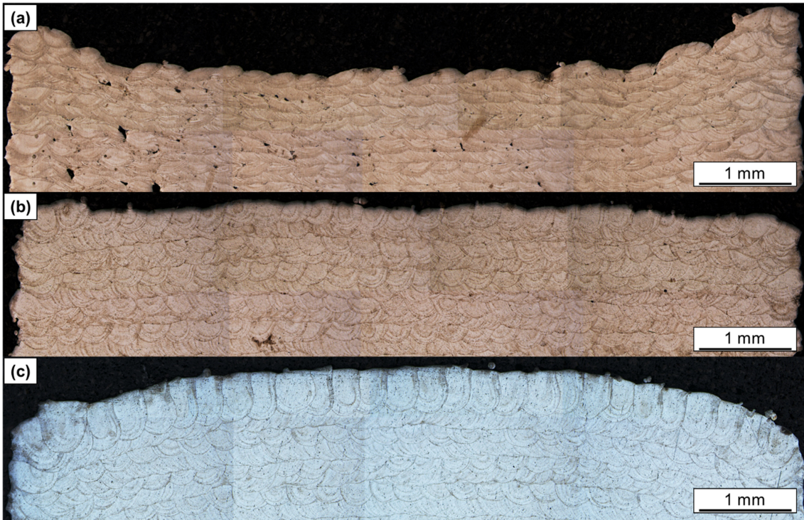
Fig. 11. OM image of the top layer (a) 600 mm/min - 110 W (b) 1,080 mm/min - 170 W (c) 600 mm/min - 220 W
